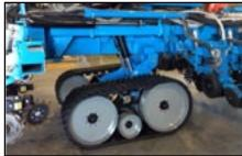
Monosem announces the new Central Lift option for select narrow-transport planter toolbars. The Central Lift option is available on planter toolbar configurations from 40' to 66'. Available with either walking tandem axle wheels or track undercarriage, the Central Lift system provides a smoother ride across uneven terrain.
